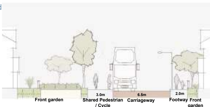
Shared Pedestrian/Cycle Route cross-section along Primary Loop Road
