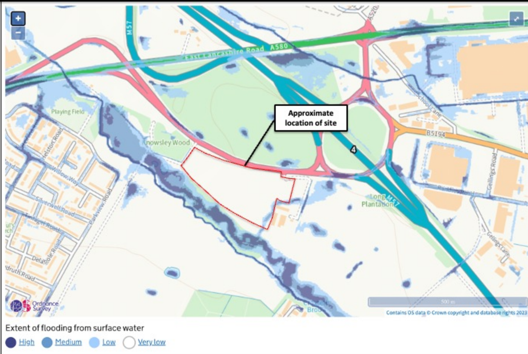
Figure 6 Environment Agency's Surface Water Flood Risk Map
