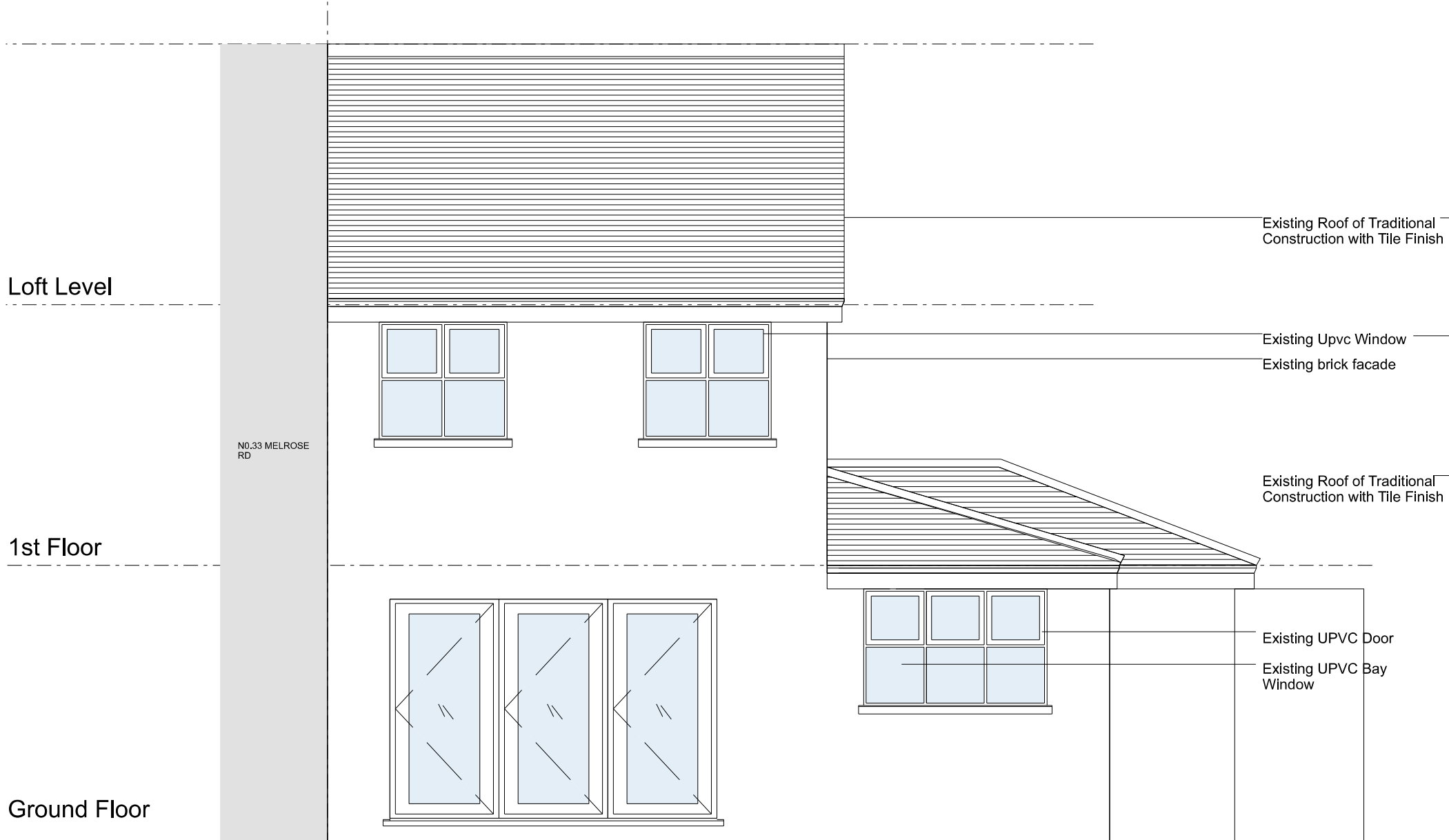
Existing Rear Elevation
