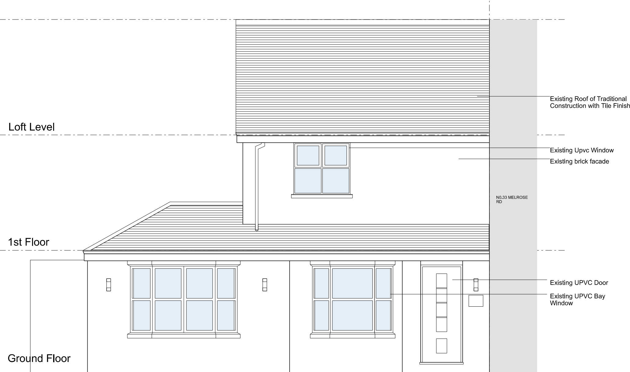
Existing Front Elevation
