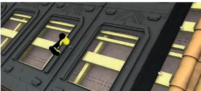
Screwing of GSE frames
