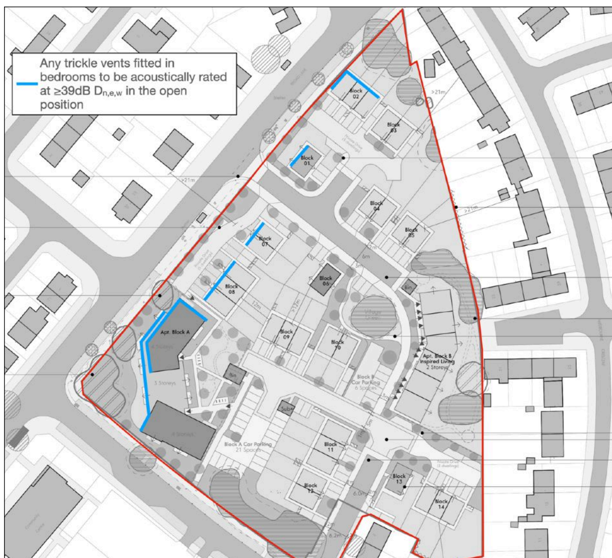
Figure 11 Recommended Noise Mitigation Scheme
