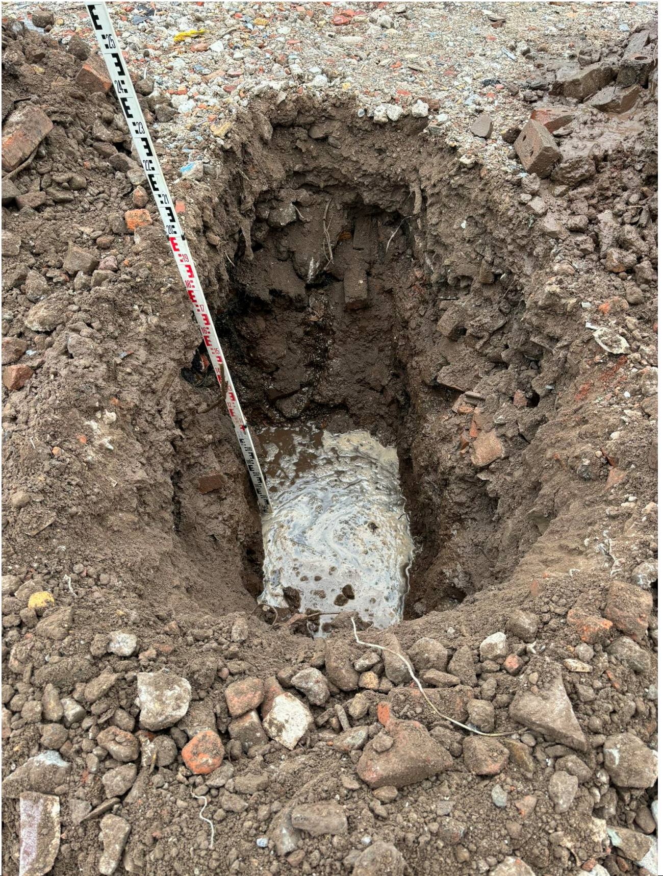
Plate 19: TP18 showing the base of the excavation and the ingress of water
