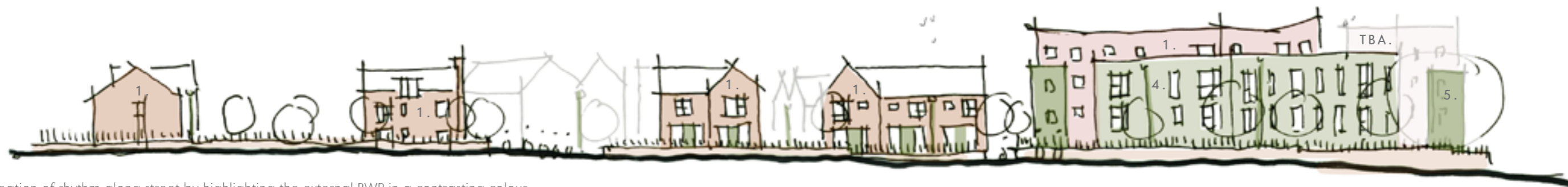
Creation of rhythm along street by highlighting the external RWP in a contrasting colour
