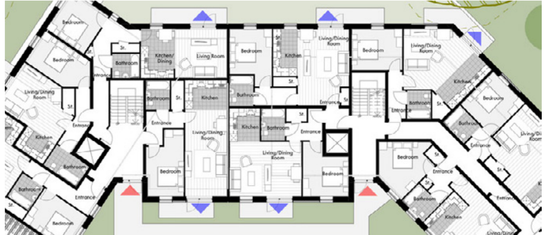
Block A - Typical Apartment Plans Ground Floor
