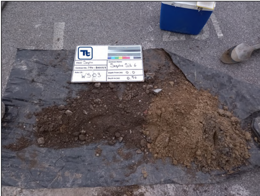
Photo Plate No. 03: WS03 hand excavated inspection pit, from 0.00mbgl to 0.90mbgl.
