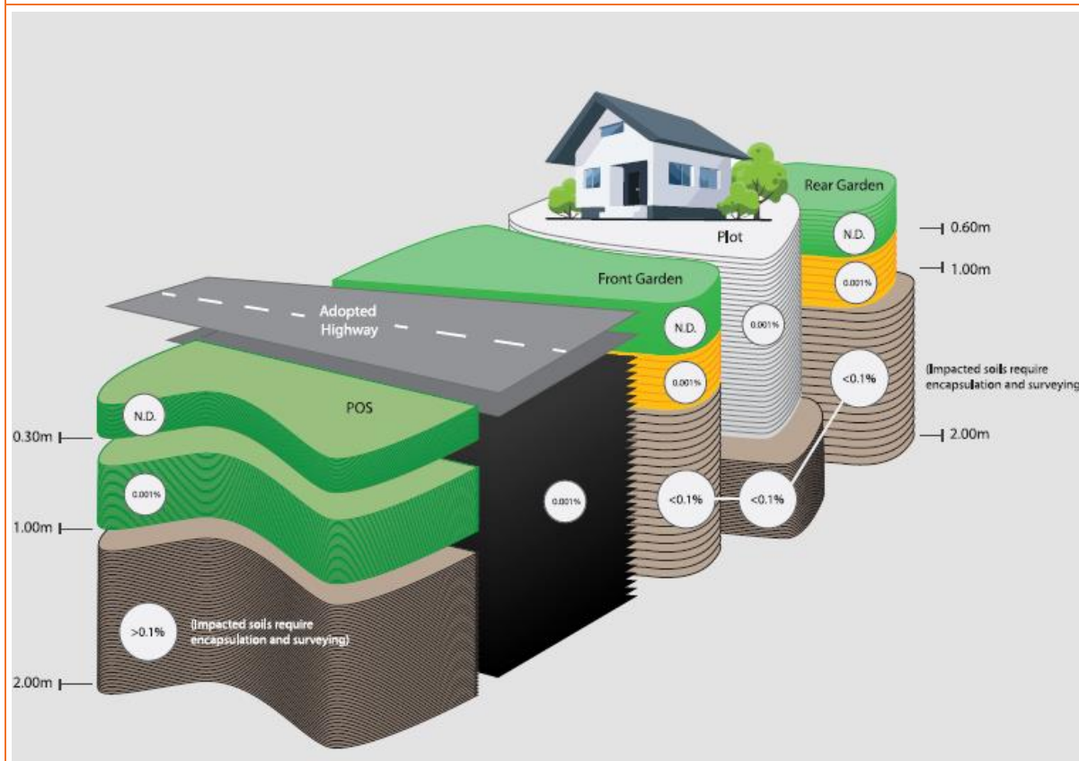
FIGURE 4.1 ASBESTOS RISK MITIGATION CONCEPTUAL SITE MODEL
