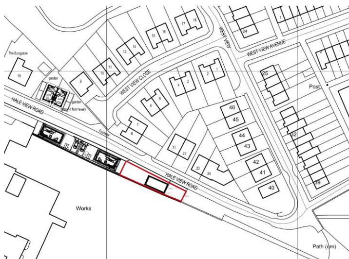
Site Plan (not to scale) illustrating the footprint of the proposed office building within the site.
