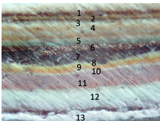
Sample 5: Lowest convex (light pink) band to fibrous cast cornice
