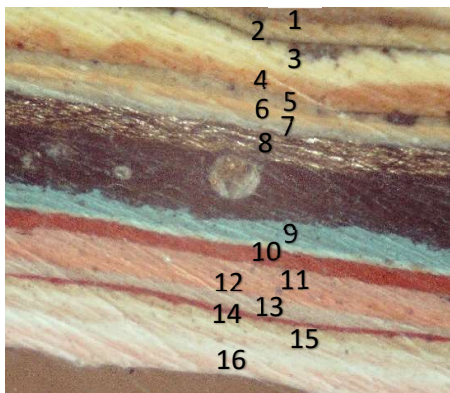
Sample 25: Central part of the fibrous plaster Keystone
