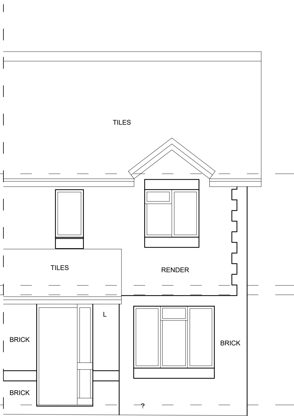
Existing Front Elevation Scale - 1:50
