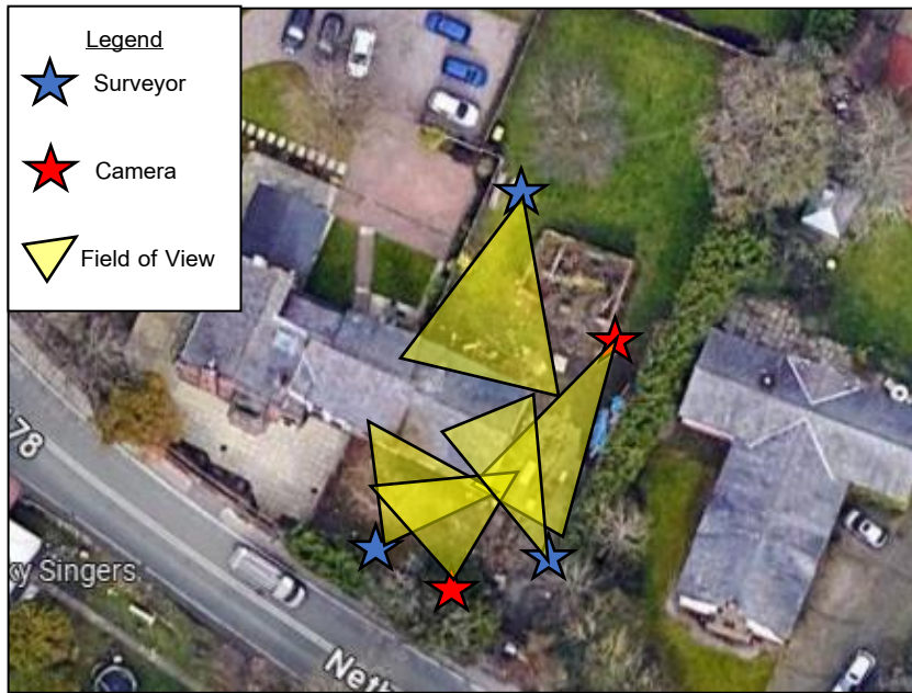
Figure 2 showing the surveyors, cameras, and field-of-view
