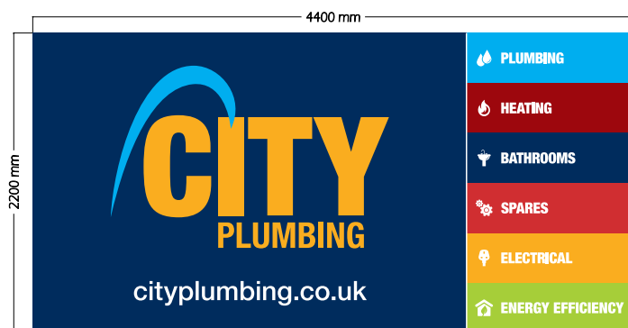
Sign 1 - 1no. Internally illuminated 89mm flex face sign finished PMS 654 Blue with digitally printed flexible face. Cap Height = 750mm HTU = 2400mm
