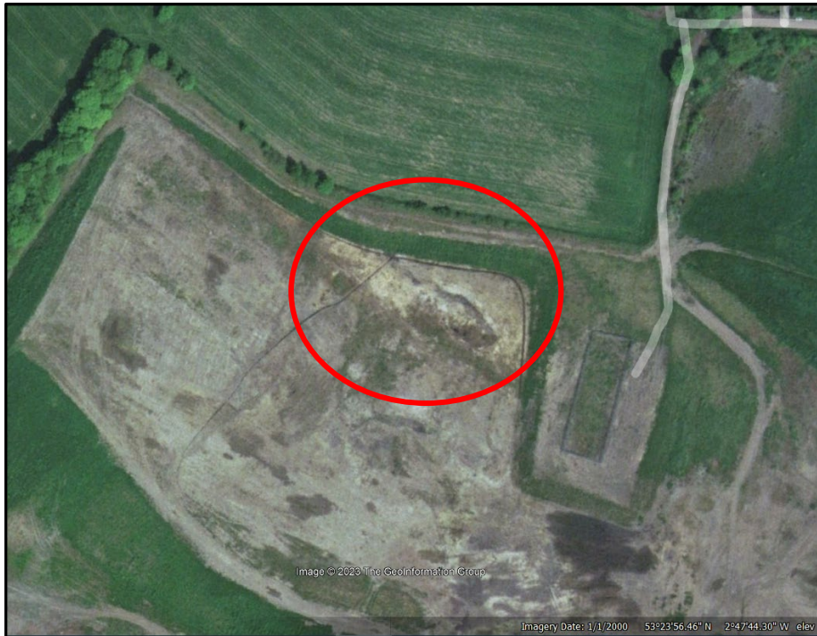
Figure 3-2 Historic Aerial Image Showing Potential Hummocky Ground
