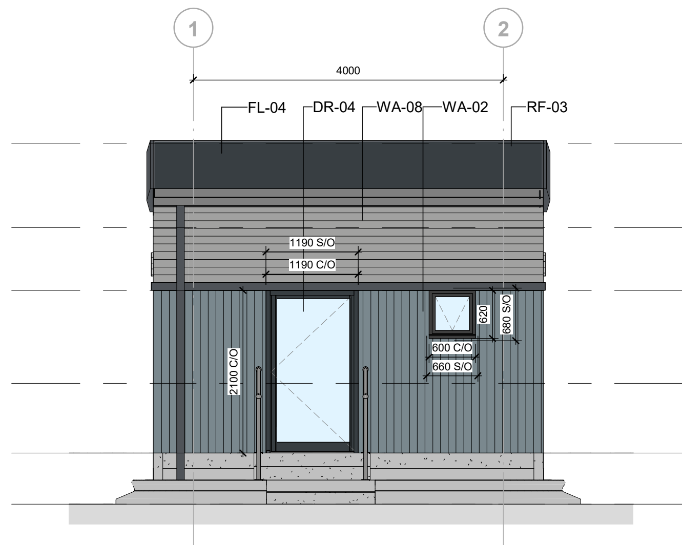
North West Elevation 1 : 50
