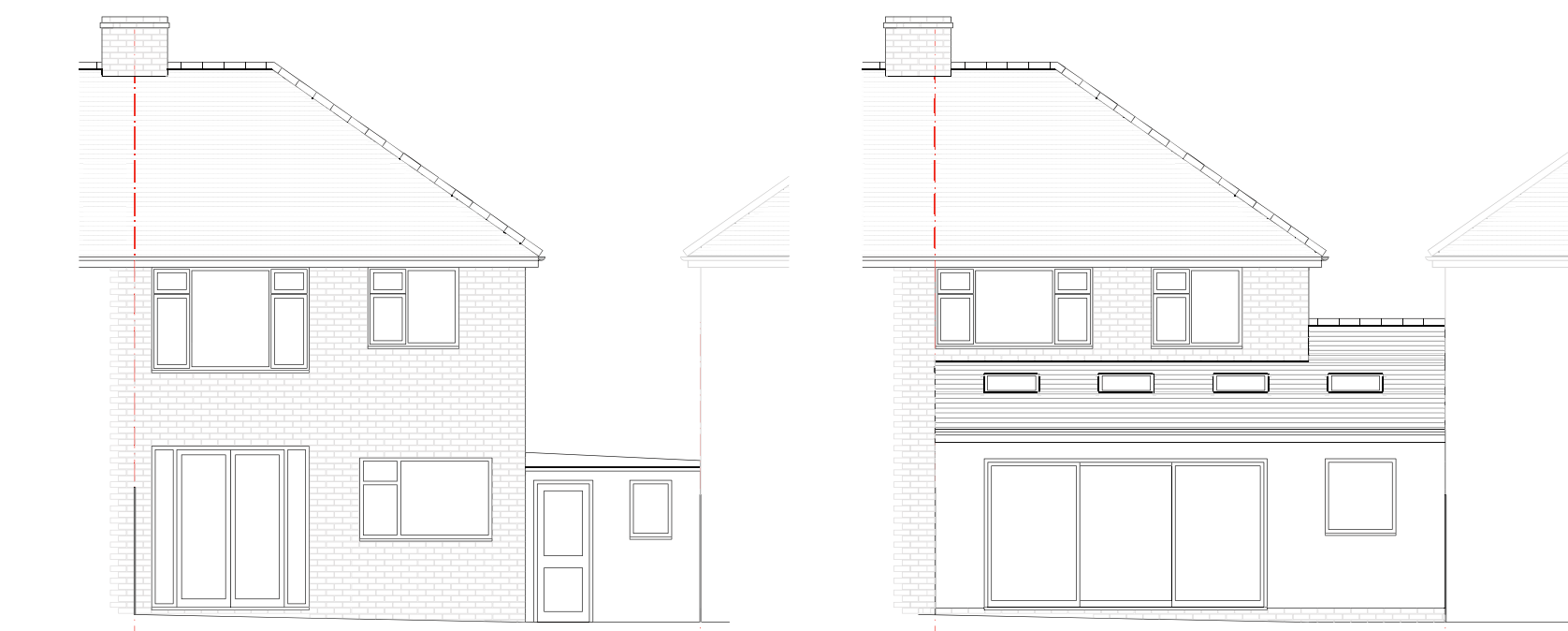
Existing South Elevation
