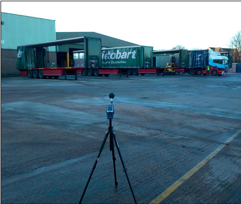
Figure 8: Measurement of forklift loading/ unloading
