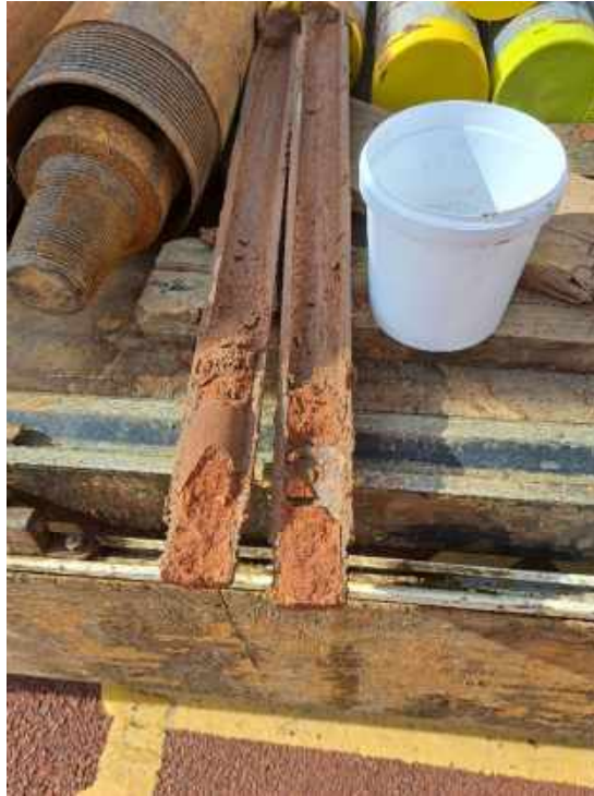
Photograph 14 Sandstone arisings from SPT at base of BH01
