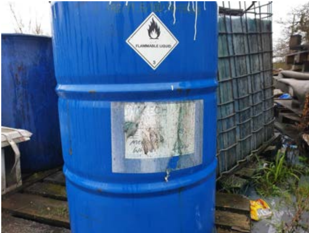
Photo 41: Close-up of blue chemical storage drum in bunded area in W of site, showing unknown contents due to poor condition label.
