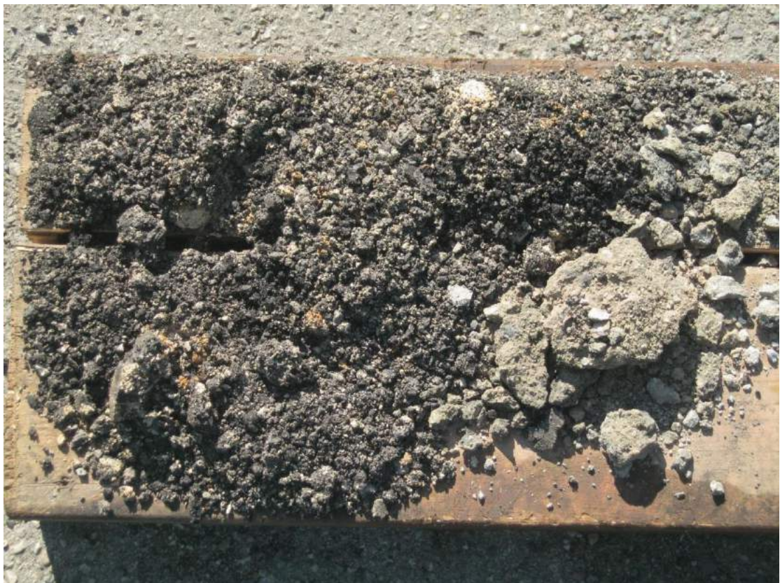
Photo 2: Made ground at WS21
