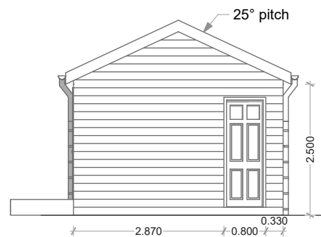
Proposed Side (NW) Elevation Scale 1:100
