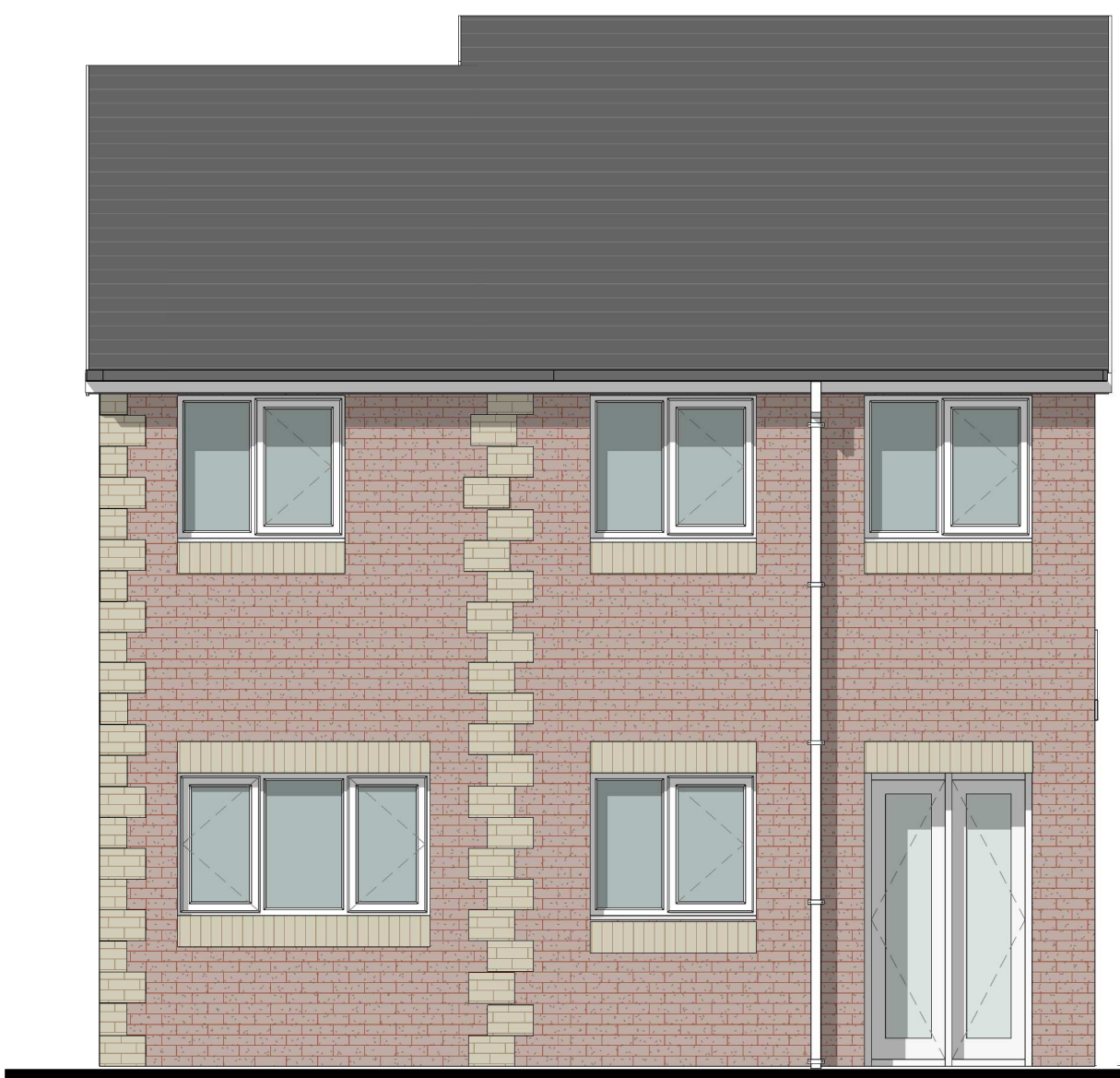
Existing Rear Elevation 1 : 50
