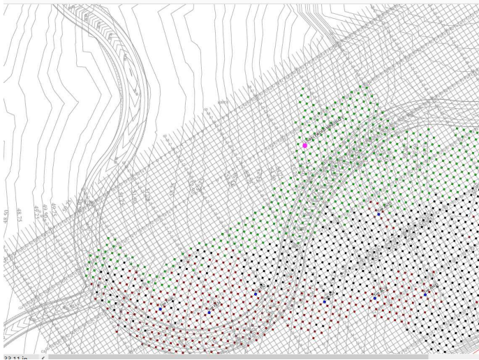
Figure 6.1 Area of Drill & Grout Pertinent to Parcel C
