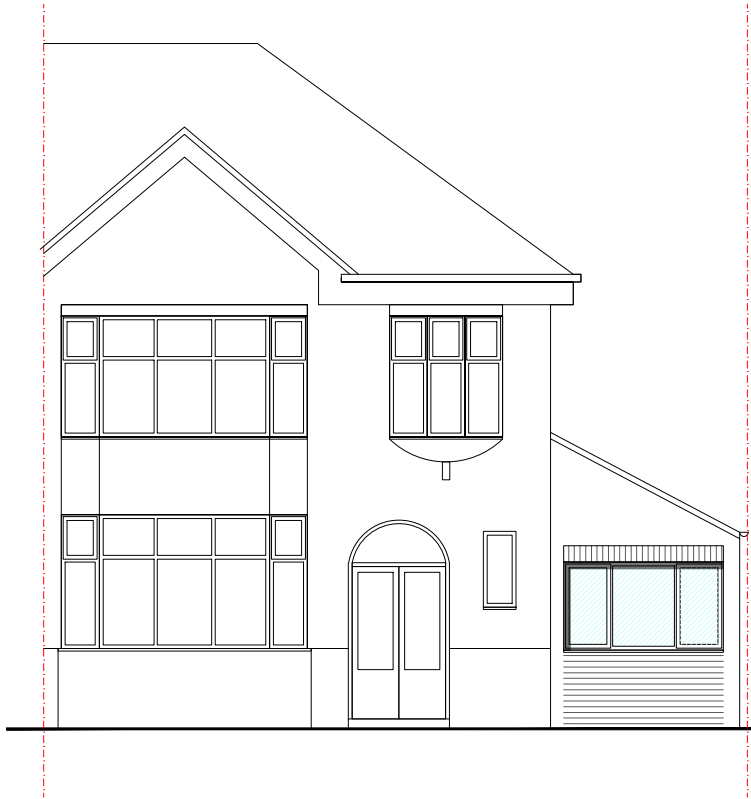
Existing Front Elevation (C) Scale 1:100
