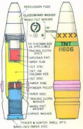
SHELL, Q.F., HIGH EXPLOSIVE, 40 MM.
