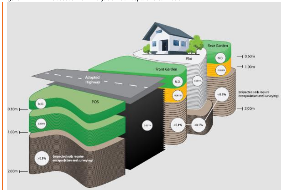
Figure 1 Asbestos Risk Mitigation Conceptual Site Model
