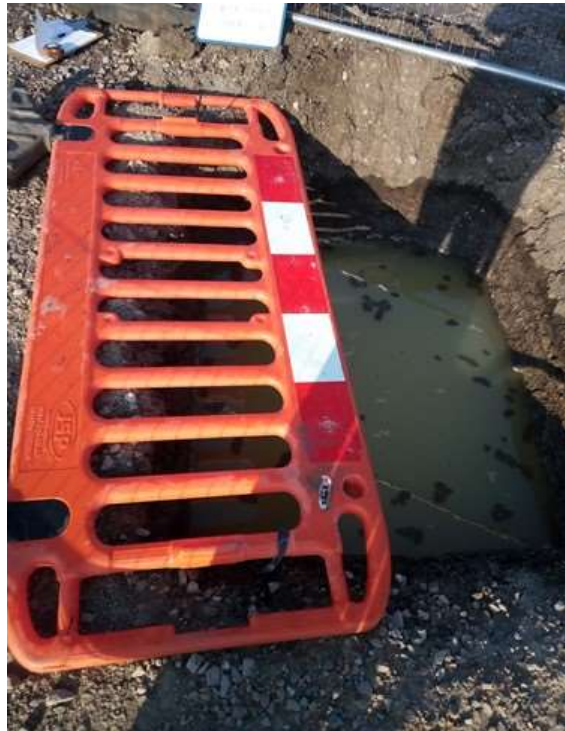
PHOTO 6 SHOWING SOAKAWAY LEVEL ON 2nd DAY
