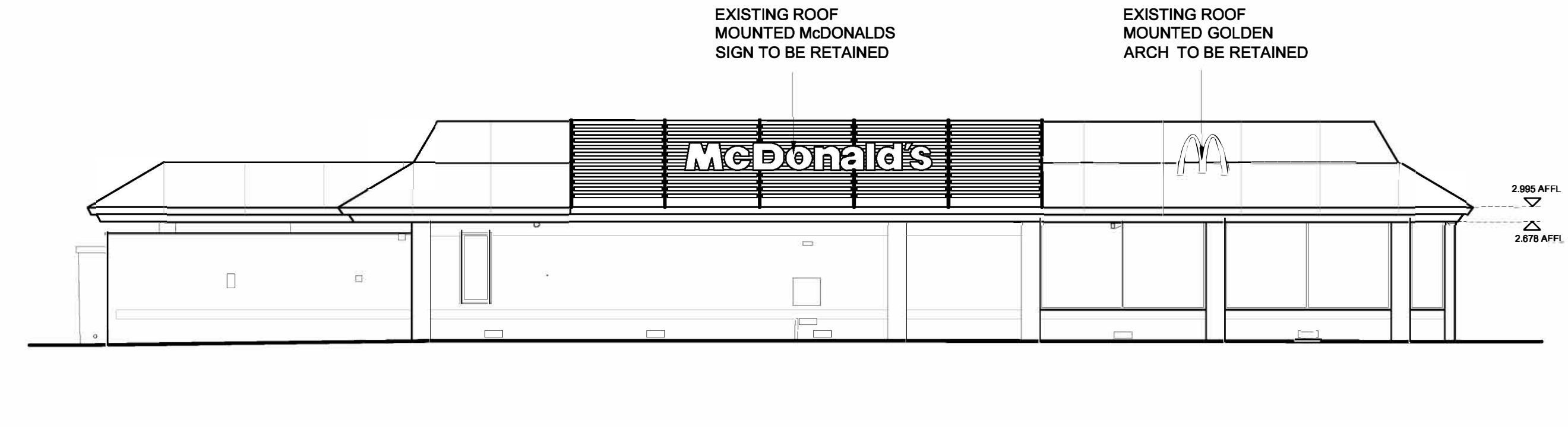
EXISTING SOUTH ELEVATION
