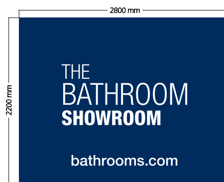
Sign 2 - 1no. Internally illuminated 89mm flex face sign finished PMS 654 Blue with digitally printed flexible face. Cap Height = 300mm HTU = 2400mm
