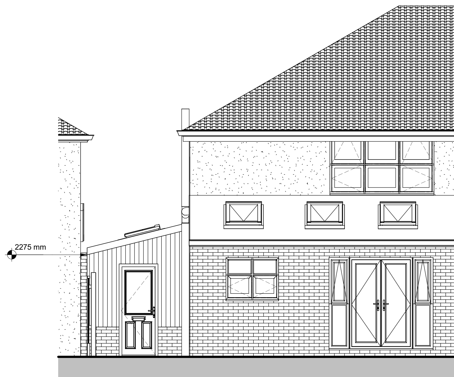
3 Rear Elevation - Existing 1 : 50
