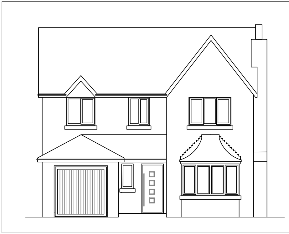
Existing Front Elevation 1:100
