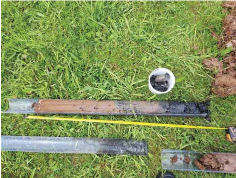
Photograph 5 WS103 deep arisings (mudstone arisings to right side of image)
