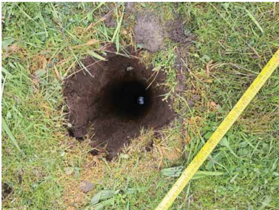
Photograph 8 WS105 inspection pit (concrete obstruction visible in base)
