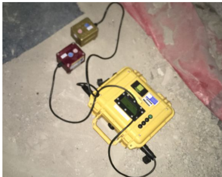
Figure 10 Vibrock Vibration Monitoring System
