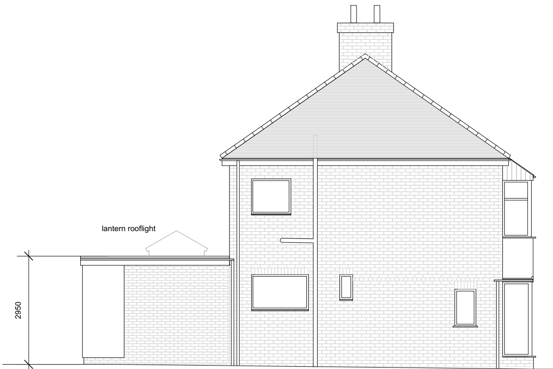
Proposed South Elevation
