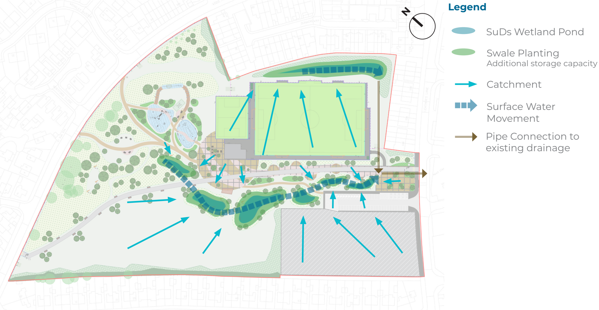
FIGURE 13: DRAINAGE STRATEGY CONCEPT DIAGRAM
