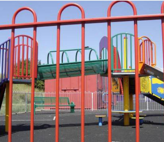
Toddler Play Area Fencing 1.2m High Anti Trap Bow Top Fencing Jackson Fencing or similar approved
