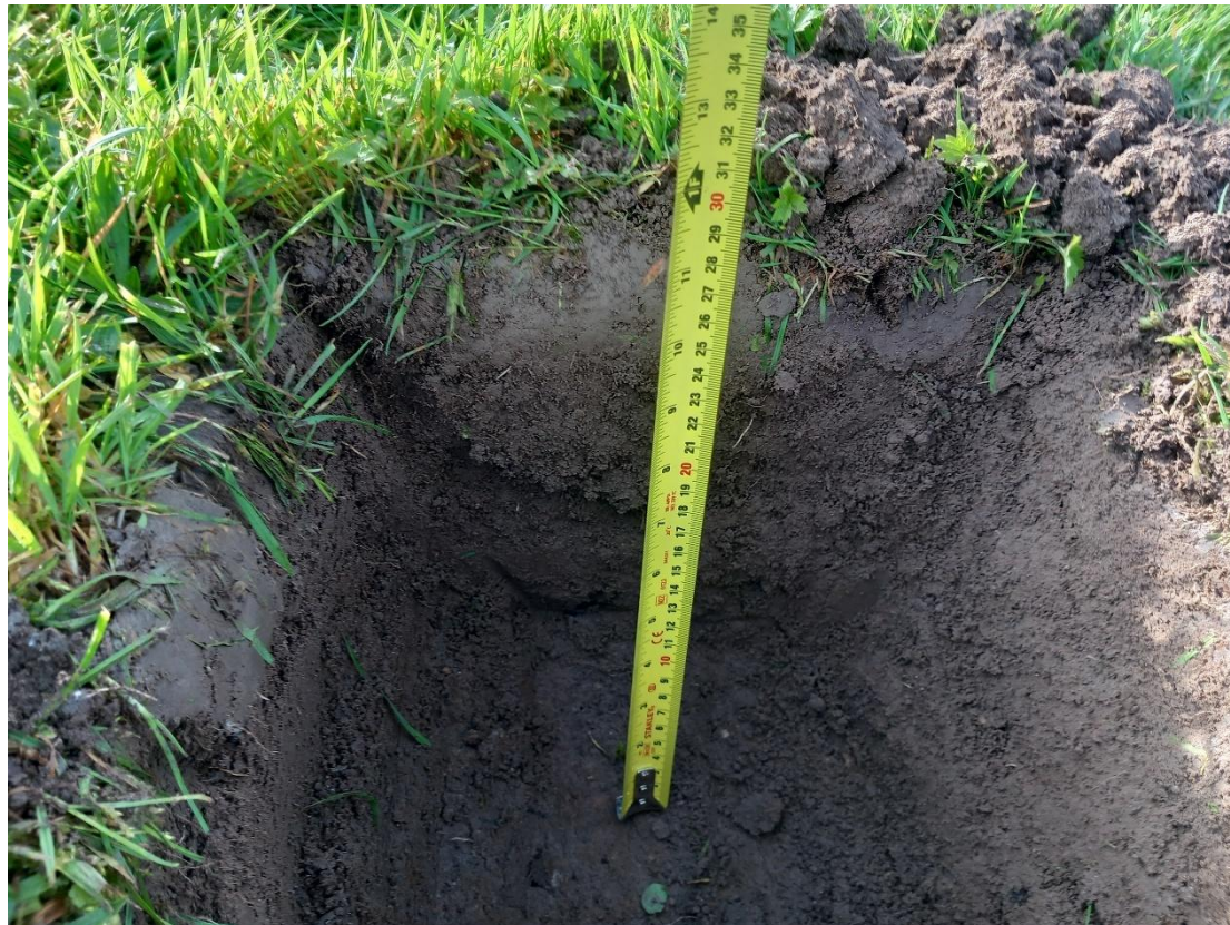
Photo 8: Excavated test pit
