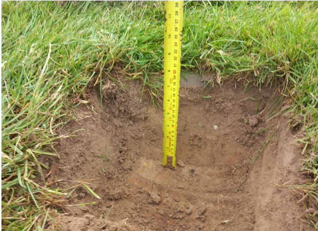
Photo 8: Excavated test pit
