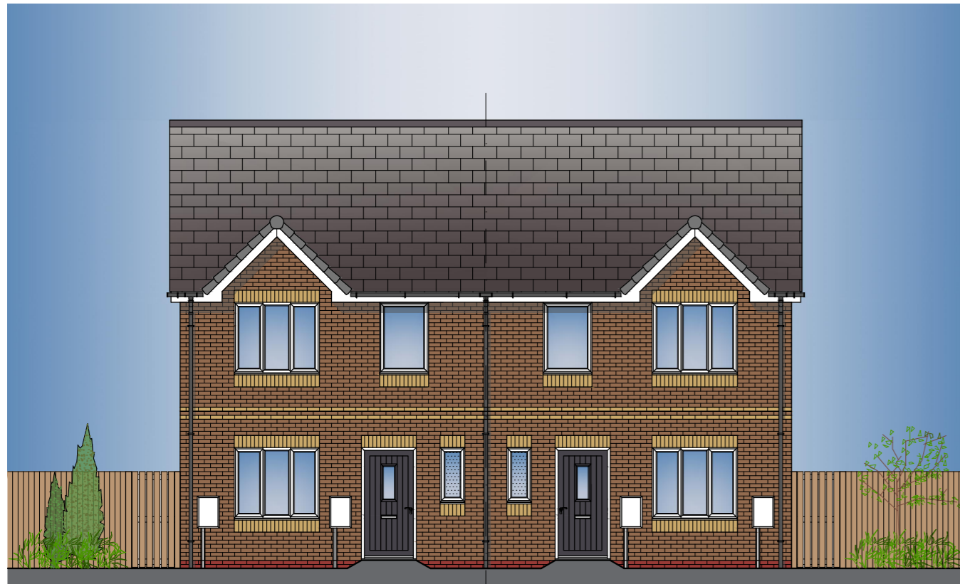
TYPE T 4B5P 100 (AS) FRONT ELEVATION - Semi-Detached
