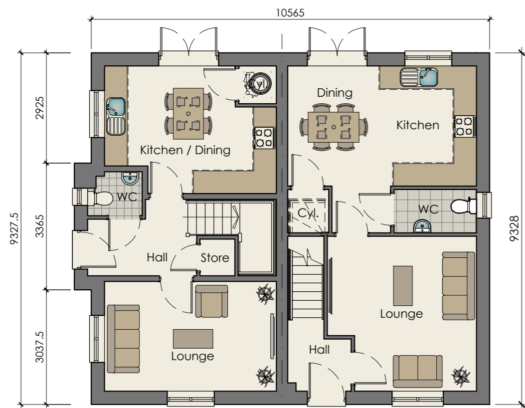
TYPE D 2B4P 81 Aspect (AS) GROUND FLOOR PLAN - Semi-Detached
