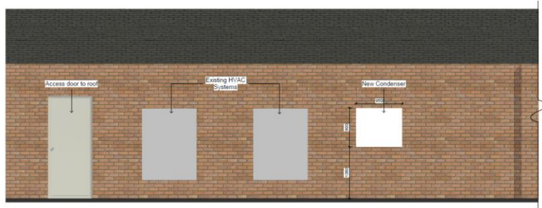
Figure 9 Proposed roof Elevation featuring proposed condenser
