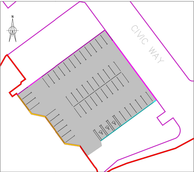
ROAD MARKINGS GENERAL ARRANGEMENT OPTION 2 - BAY DIMENSION = 5.0m x 2.6m. 43 PARKING BAYS ACHIEVED PLUS 3 DISABLED PARKING BAYS ACHIEVED SCALE 1:250
