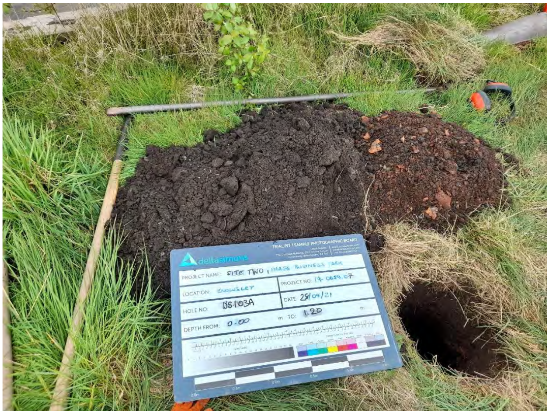
Photograph 20 – DS103A 0.0 to 1.2 m.
