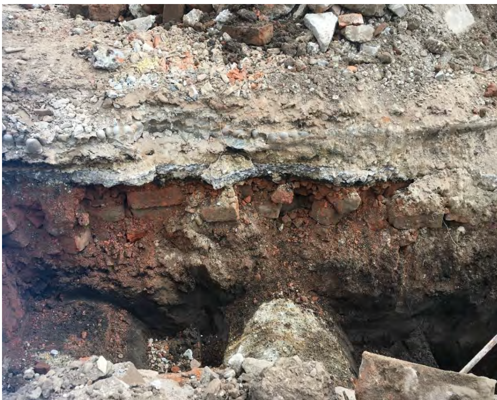
Photograph 9 – Brick and concrete obstruction in TP103 at 0.65 m bgl.
