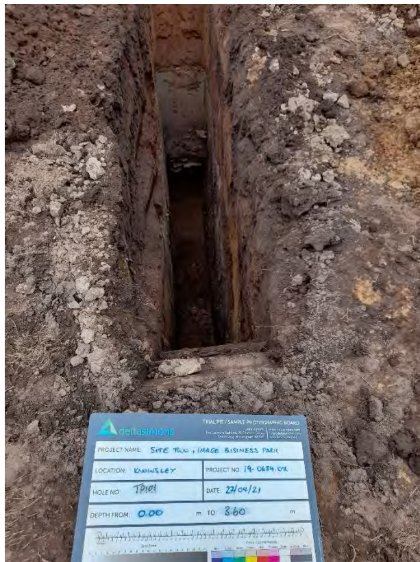
Photograph 1 – TP101 Trial Pit 0.0 to 3.6 m.
