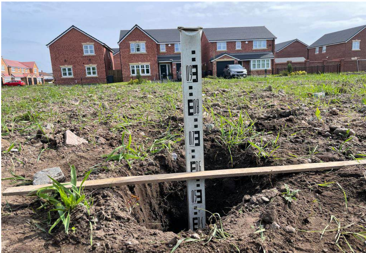
PLATE 4 – Depth of Soil Cover in IP2 (~600mm) @ May 2022.
