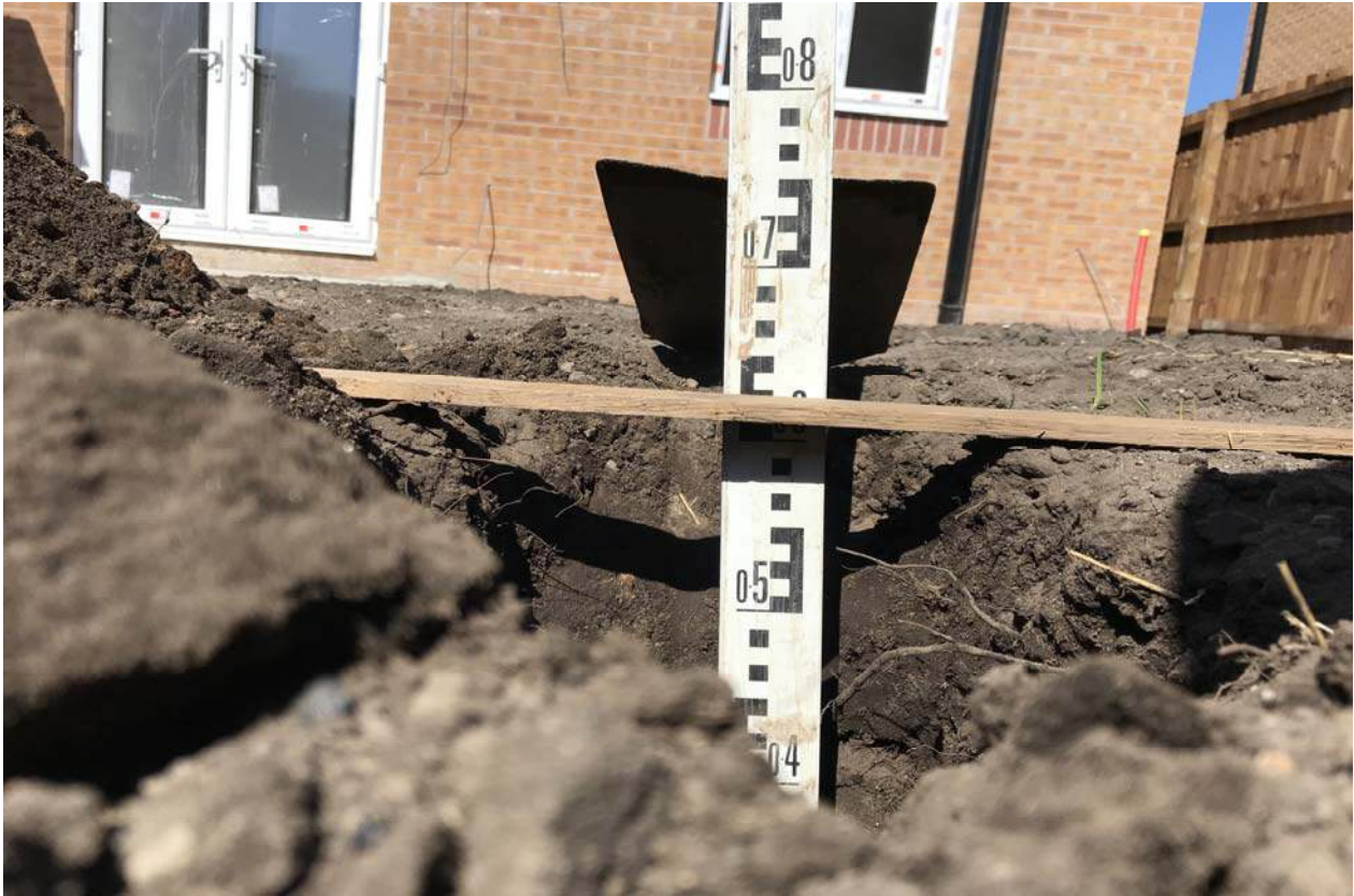
PLATE 5: Depth of soil cover in Plot No.79 (615mm)
