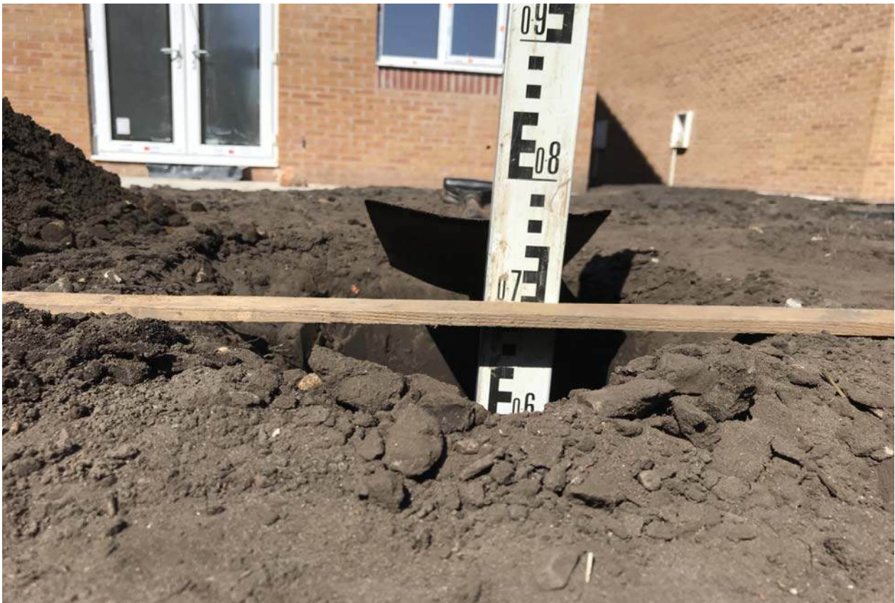
PLATE 8: Depth of soil cover in Plot No.80 (690mm)
