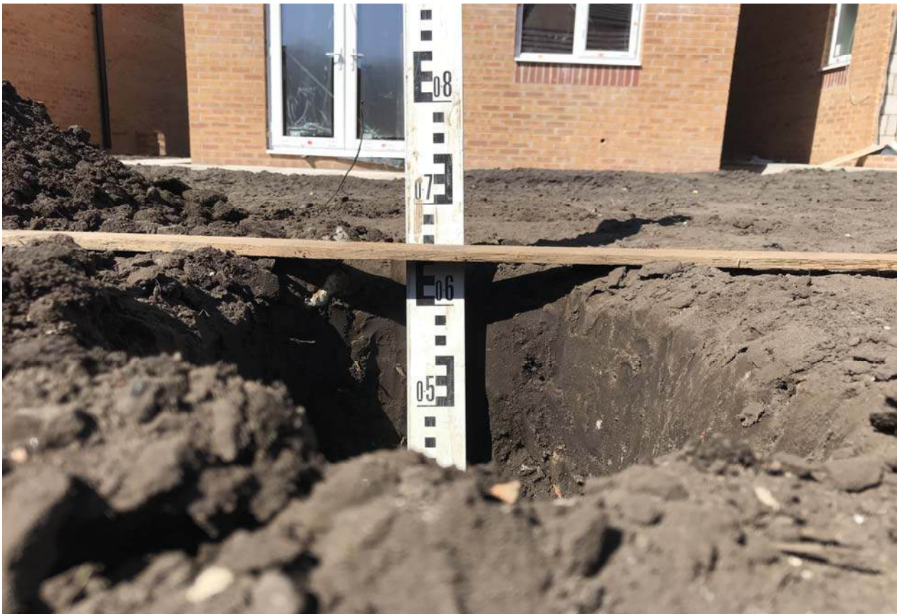
PLATE 10: Depth of soil cover in Plot No.81 (650mm)
