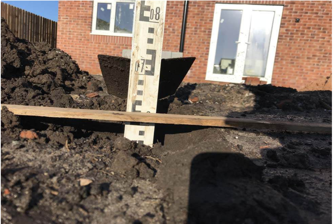
PLATE 5: Depth of soil cover in Plot No.70 (610mm)
