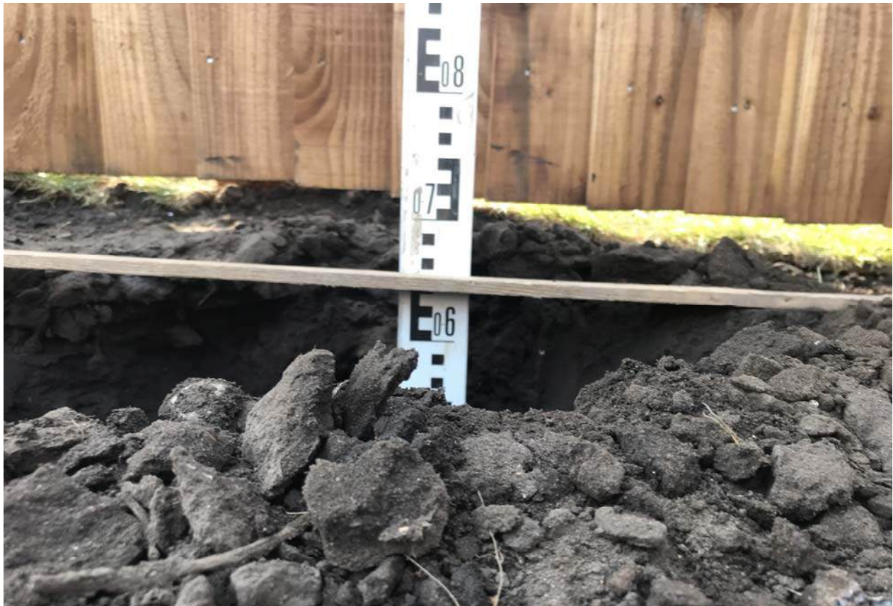
PLATE 3: Depth of soil cover in Plot No.78 (650mm)
