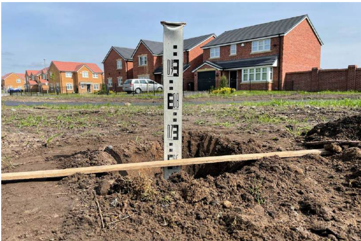
PLATE 2 – Depth of Soil Cover in IP1 (~620mm) @ May 2022.
