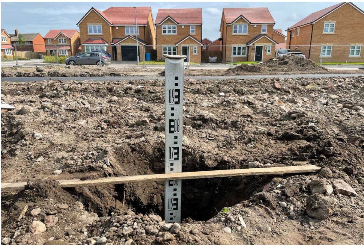
PLATE 8 – Depth of Soil Cover in IP4 (~630mm) @ May 2022.
