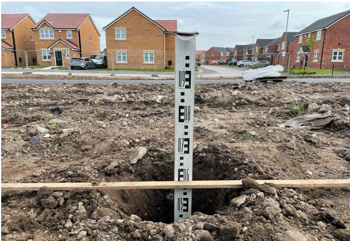
PLATE 6 – Depth of Soil Cover in IP3 (~600mm) @ May 2022.
