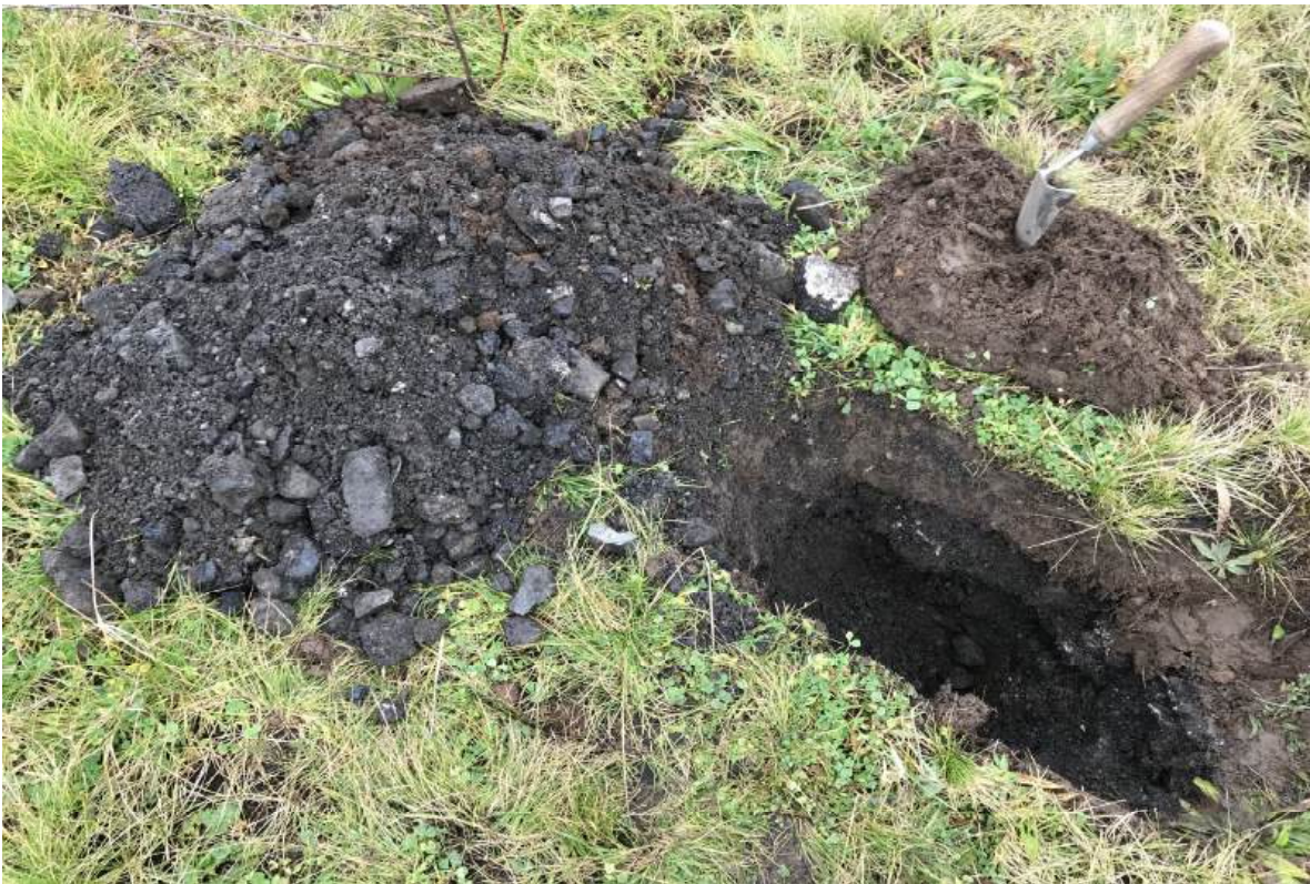
PLATE 6: Supplementary sampling of made ground in TP107
