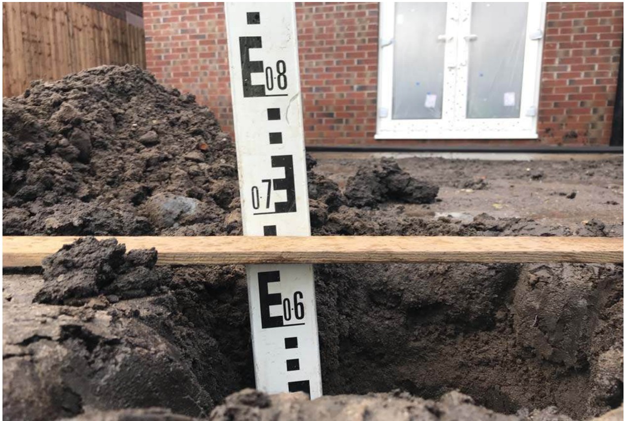
PLATE 5: Depth of soil cover in Plot No.55 (665mm)
