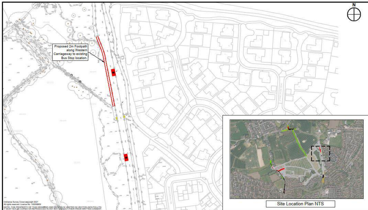
Figure 5.3: Queensbury Way – PRow Proposed Pelican Crossing
