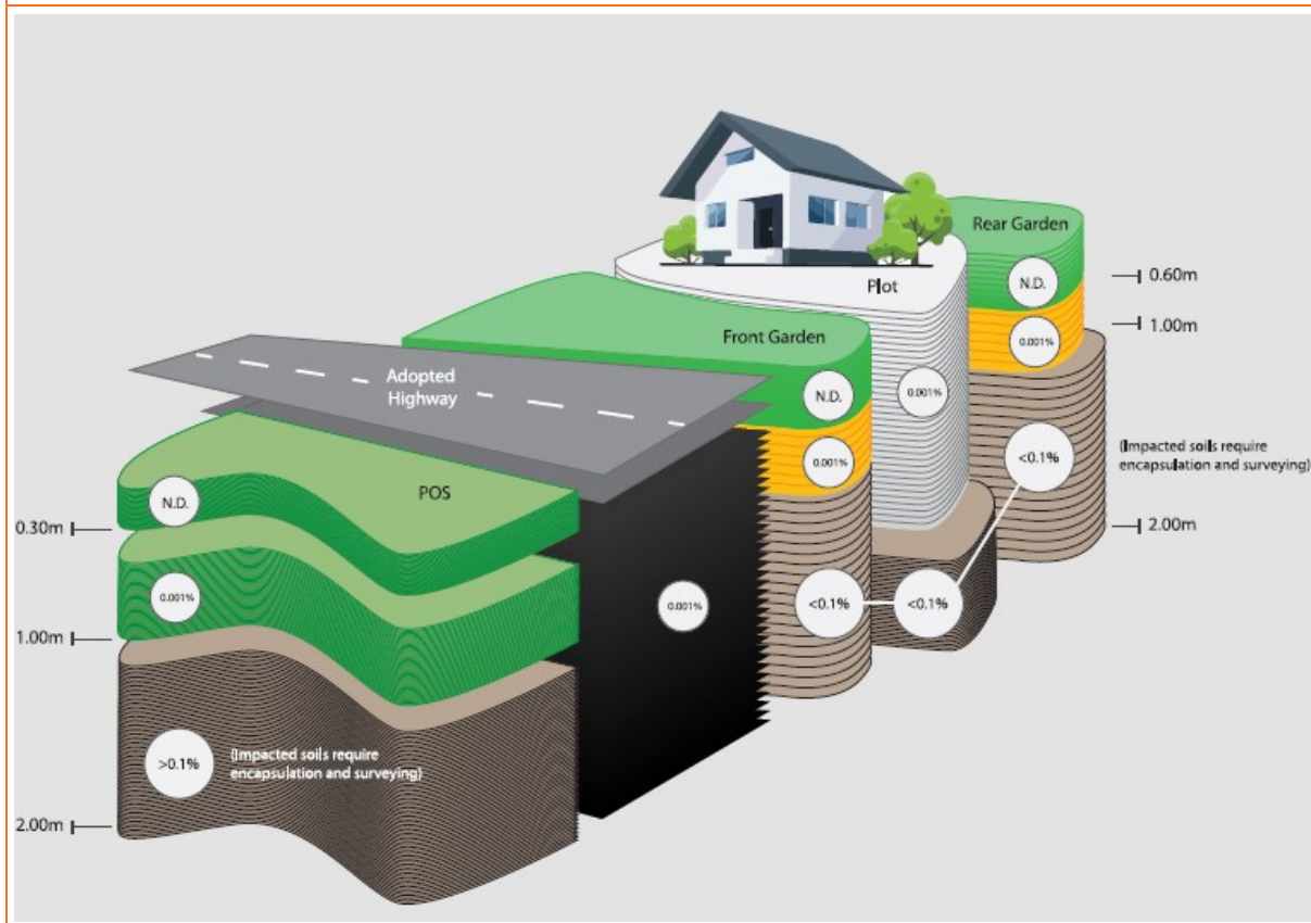
FIGURE 4.1 ASBESTOS RISK MITIGATION CONCEPTUAL SITE MODEL
