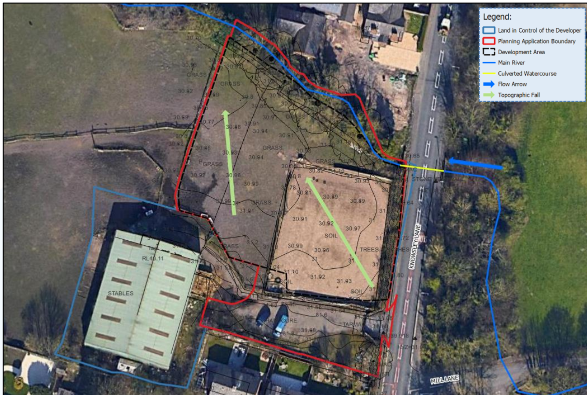
Figure 1: Existing Drainage Plan (Betts Hydro, 2023)
