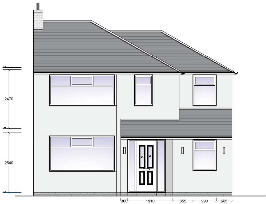
PROPOSED FRONT ELEVATION (Scale 1:100) SCALE BAR - (mm) 500 1000 2000
