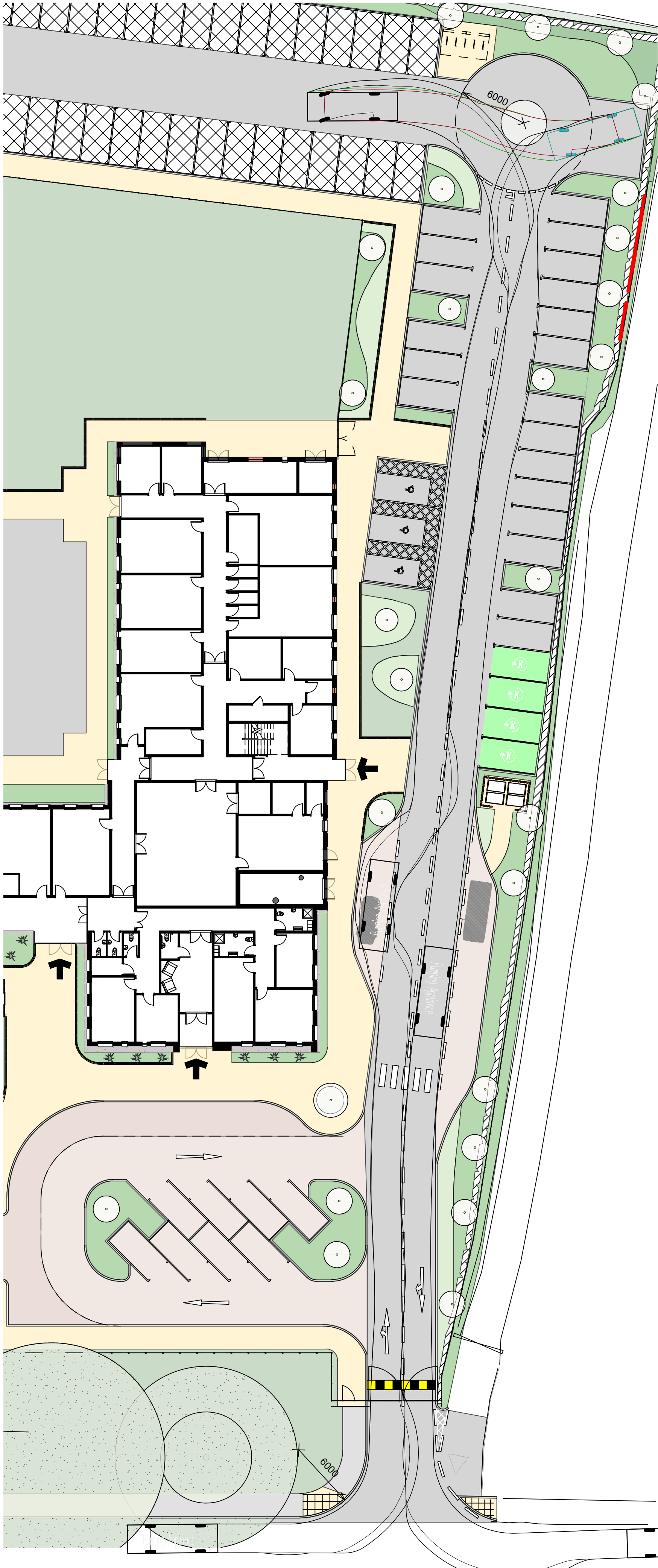
Fire Appliance - Layby and Turning Head
